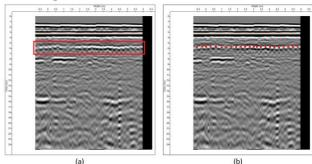
Figure 3: Example of dowels on a transverse joint, (a) highlighted by the red square and (b) identified singularly by the red dots.
