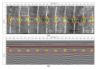
Figure 4: Example of dowels on longitudinal joints from above (a) and in a longitudinal profiles (b); in both figures, the dowels are highlighted by the red square while the green circles highlight the transverse joints.
